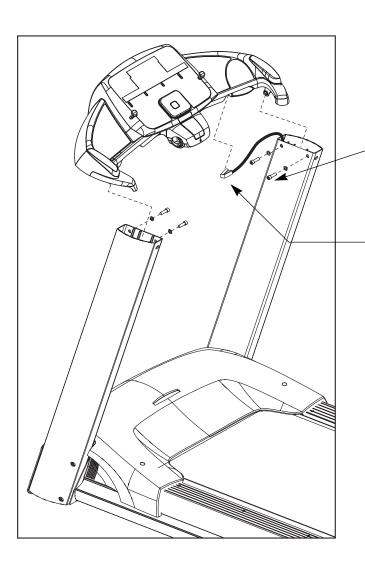
Attach the display console using four socket head screws (G) and four washers (D). Align the mounting holes and insert all four fasteners with your fingers. Tighten the fasteners on one upright before performing the same step on the opposite upright. Push down on the edge of the display console to close the gap between the console and the upright and then wrench tighten the fasteners.
